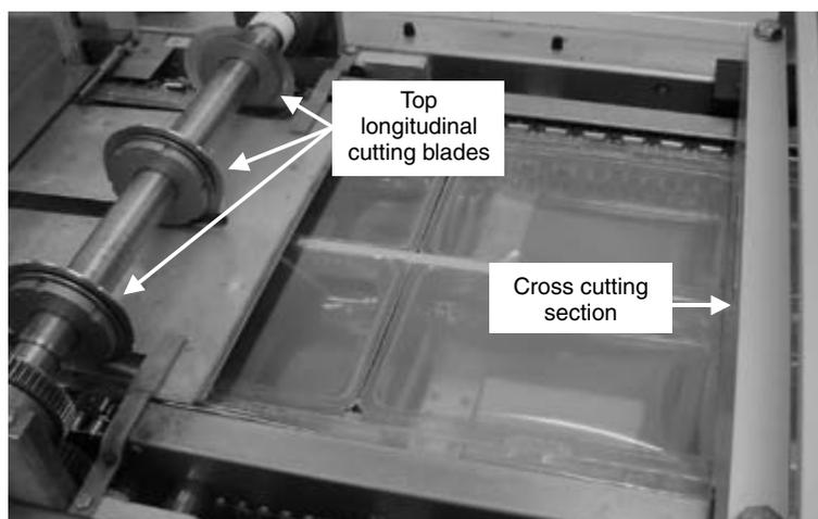
**Figure 10.11** Cutting section on the Multivac R230.
