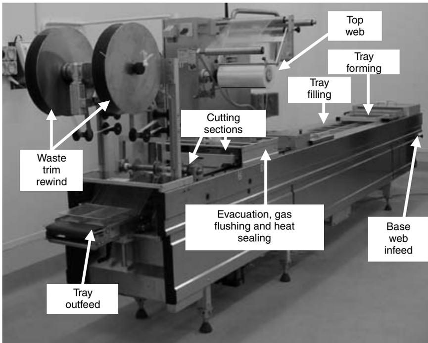
**Figure 10.7** Multivac R230 thermoform fill seal machine.
